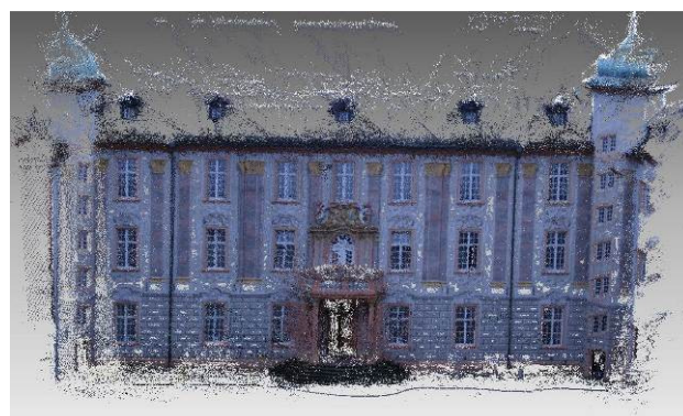
Figure 8. DSM of one of the façade of the inner courtyard of the Ettlingen castle.
