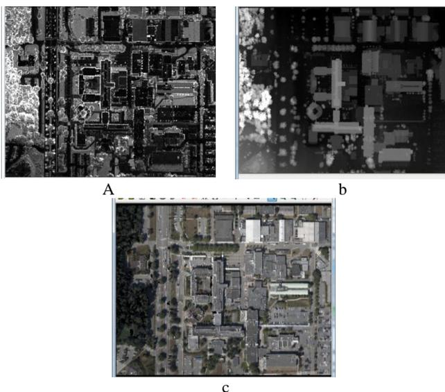
Figure 4: Geometrically Calibrated and Radiometrically corrected Intensity Image (a), DSM (b), and Ortho-rectified Aerial Photo (c)
