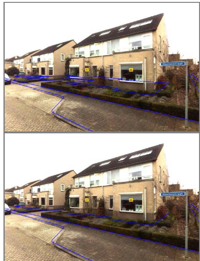
Figure 12. Hidden line removal from 2D base map data
