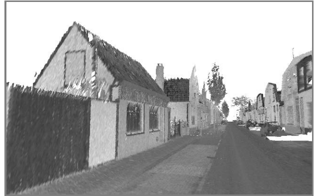
Figure 3. A triangle mesh generated from a LiDAR point cloud
