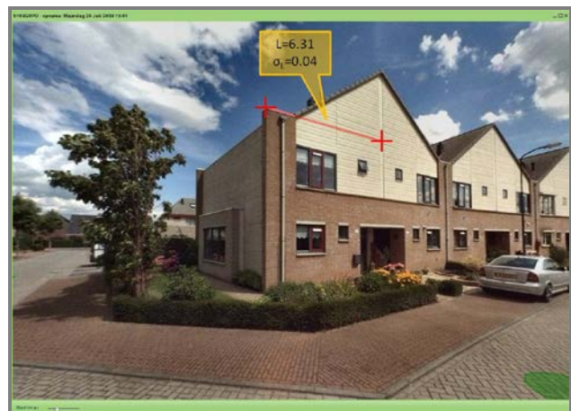
Figure 7. Example of line measurement in a single image
