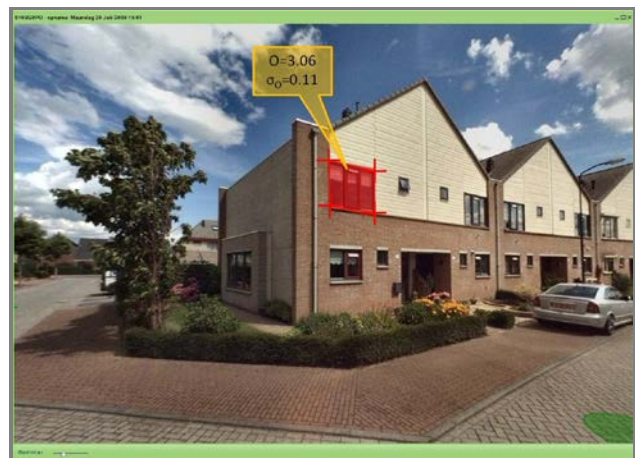
Figure 8. Example of area measurement in a single image
