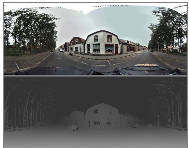
Figure 4. An example of a panoramic image and a grayscale representation of its corresponding depth layer
