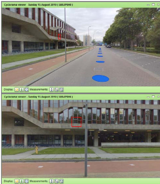
Figure 5. Navigation through Depth Cycloramas using depth data to identify a façade, represented by the rectangle cursor: a double click in the top window results in a jump to the picture shown in the bottom window.
