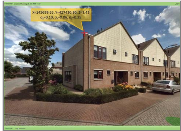
Figure 6. Example of point measurement in a single image
