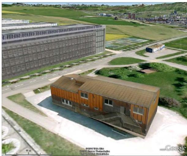
Figure 13. 3D-Model derived from UAV images of the HXE-building at Campus Science City ETH Hoenggerberg, imported to Google Earth
