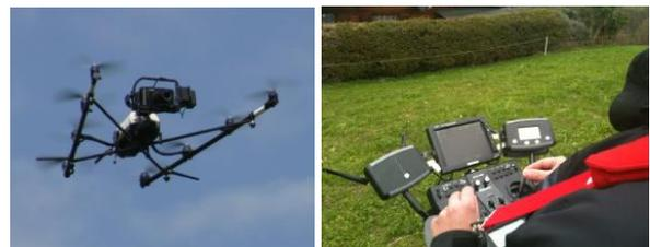
Figure 3. Used UAV system: Octocopter Falcon 8, AscTec
