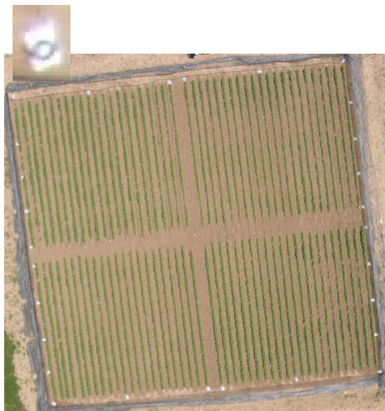
Figure 3. RGB field experiment image with targets to georeference. In the left up corner a detail of a target.
