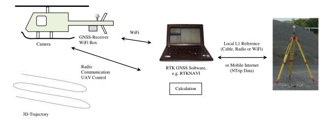
Figure 4. RTK GNSS Low-cost System based UAV-Control
