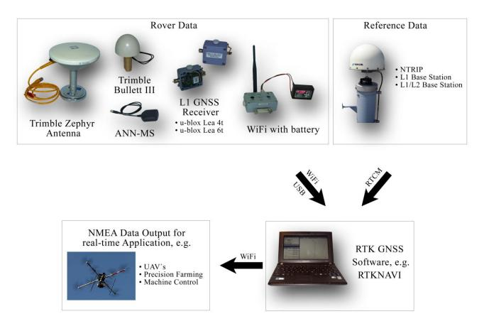
Figure 2. RTK GNSS Low-cost System Components
