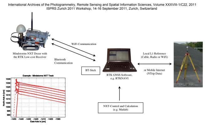
Figure 1. RTK Mindstorms NXT-Control via the RTK GNSS Low-cost System
