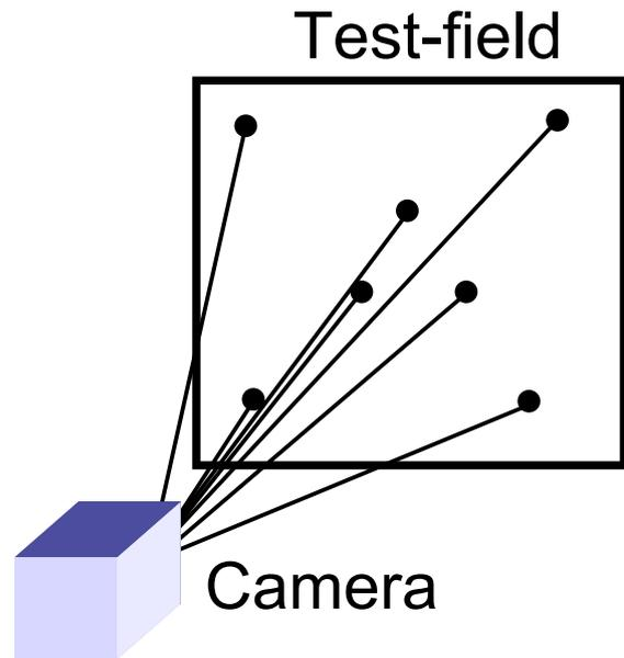
Figure 1: Schematic of the test-field calibration setup
