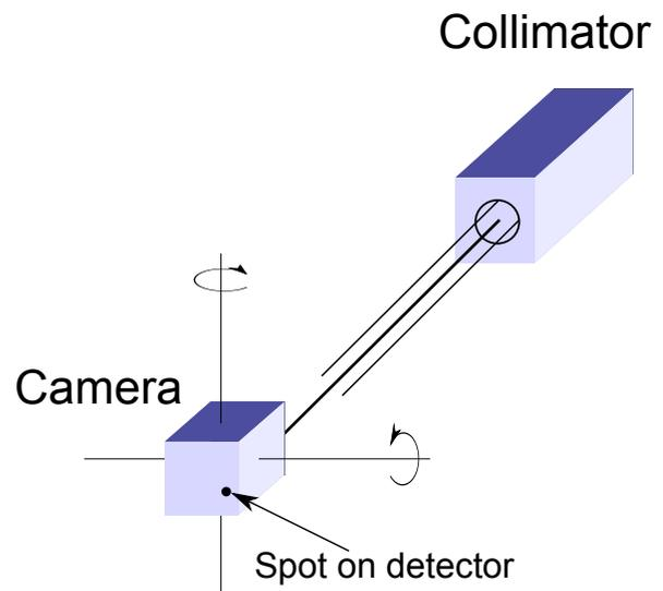
Figure 2: Schematic of the goniometric calibration setup
