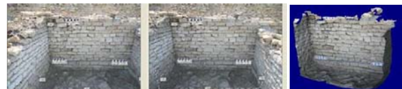
Figure 9. Canon EOS 5D with 28mm focal length: stereopair (left) and 3D textured model from matching (right).
