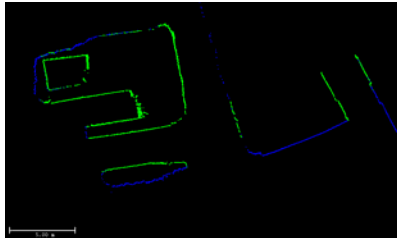
Figure 11. Horizontal section of the southern part of the theatre coloured by cloud: green for the image based point cloud and blue for the TLS point cloud.
