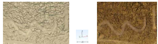
Figure 5. Visualization of the sub-millimetric meshed model (250mm x 160mm) of a clay panel recorded with the FARO ScanArm, with textures (right)
