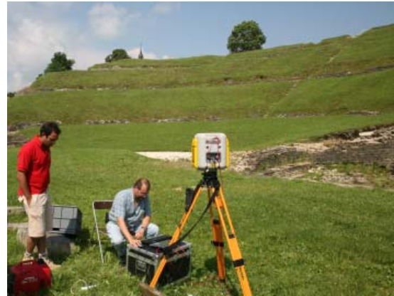
Figure 7. Positioning of the Trimble GX TLS at the ground level of the theatre of Mandeuire.
