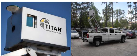
Figure 1. TITAN mobile laser scanning system.
