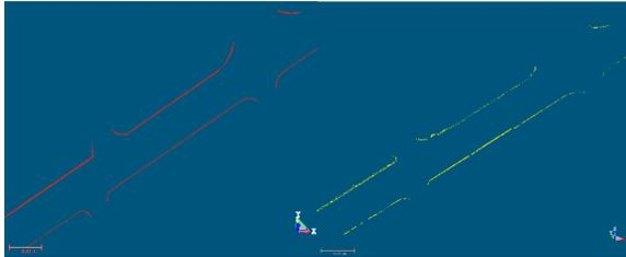
Figure 14. The road curb of Auriga Dr. Left: truth data. Right: the extracted curb.
