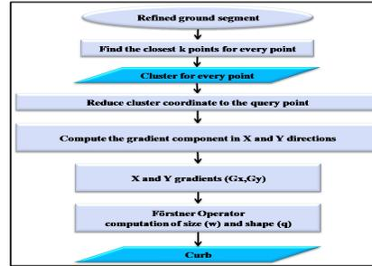
Figure 5. Curb extraction pipeline.
