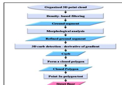
Figure 4. Street floor extraction pipeline.
