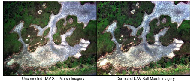
Figure 11: Visual comparison of the improvements by the application of sensor corrections and radiometric calibration (Image Bands Coregistered).
