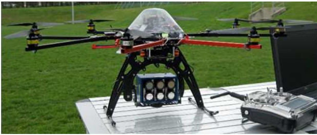
Figure 1: MikroKopter Oktokopter with mounted mini-MCA Multispectral Sensor (Photo: Darren Turner)
