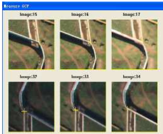
Figure 5 Measuring GCP in MAP-AT
