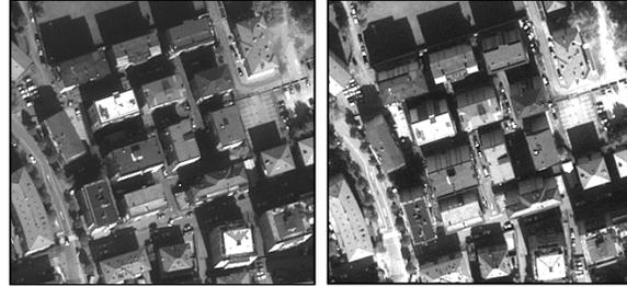
Figure 7. Example of occlusion between tall buildings in GE1 stereo-pair: forward view [left] and backward view [right].
