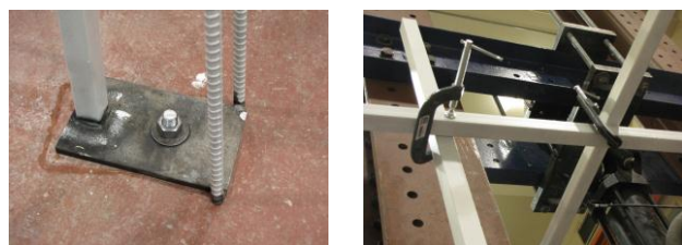
Figure 3. Part of the metal frame built to hoist the cameras and projectors of the digital photogrammetric system
