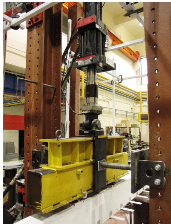
Figure 1. Spreader beam (in yellow) attached to a hydraulic actuator (in black and silver)
