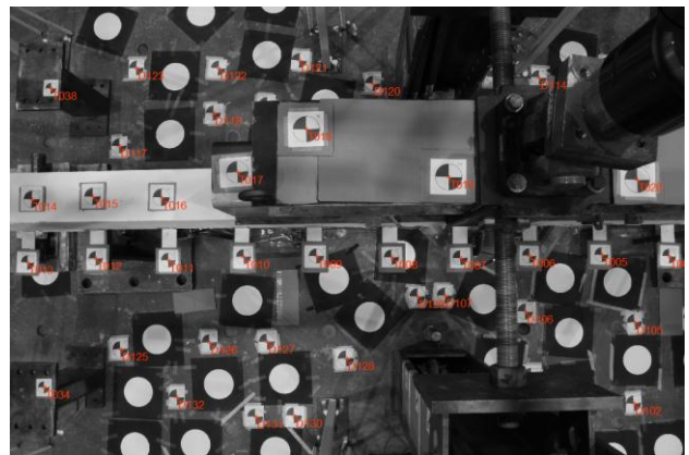
Figure 5. Example of the distribution of signalized targets on the floor, the concrete beam, and the spreader beam for the relative orientation estimation before the static loading case
