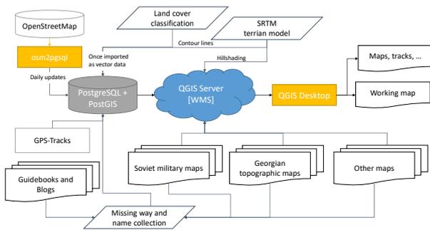
Figure 1. Parts of the WMS for the mapping project show the implemented geodata integration into the service.
