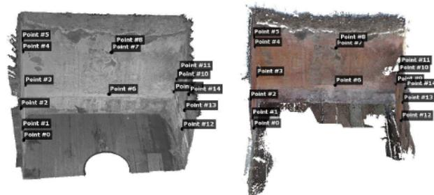
Figure 5. GCPs chosen on the laser scanner point cloud (on the left) and corresponding points on the photogrammetric point cloud (on the right).
