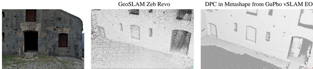
**Figure 11.** A close up view of the main entrance of Batteria di Mezzo fort in Riva del Garda, Italy (left) and the two point clouds of its facade, surveyed with the GeoSLAM Zeb Revo (middle), and the proposed prototype (right), respectively.
