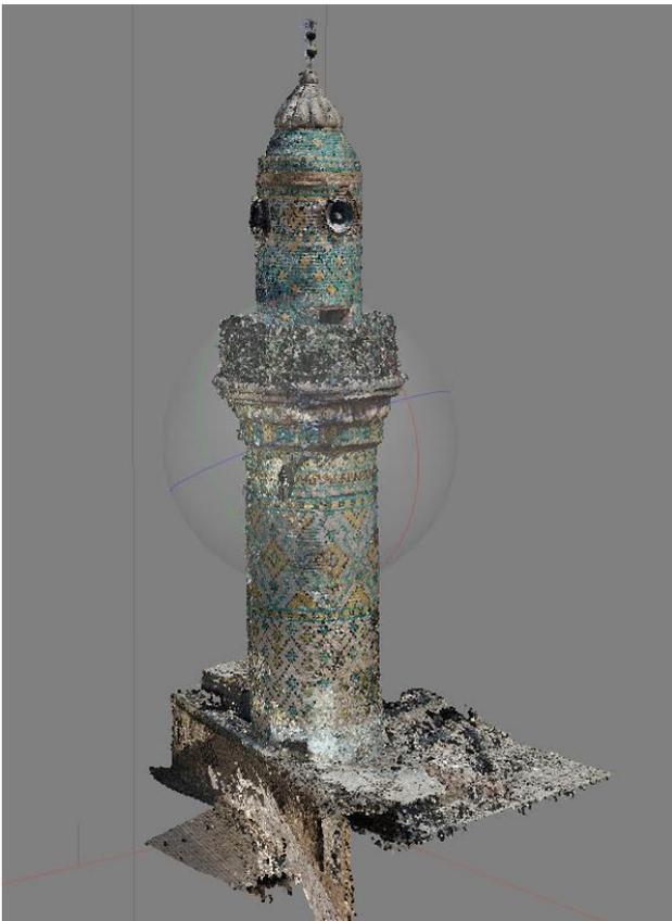
Figure 5. Raw uncleaned point cloud from photogrammetric data in Agisoft Metashape wasn't suitable for precise processing. Until the merging with the laser data yielded very good results.
