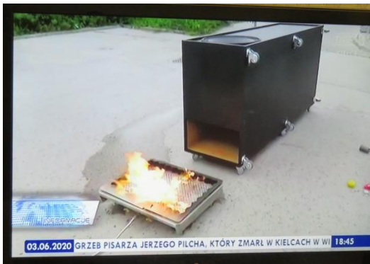
Figure 1. Extinguishing flames with the use of the prototype of the high-power acoustic extinguisher (TVP, “Informacje” from 03.06.2020).
