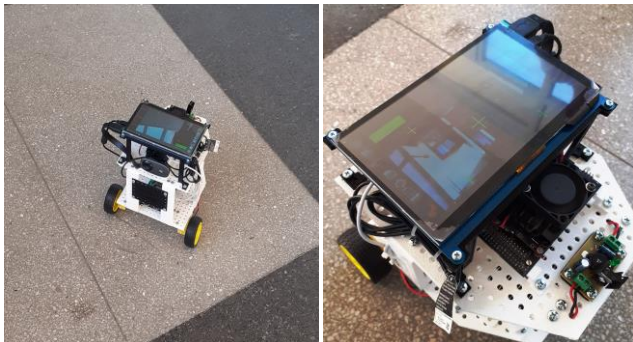
Figure 3. A mobile robot that detects flames and smoke using deep neural networks.
