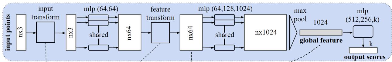
Figure 4. PointNet classification architecture (Qi et al., 2017)
