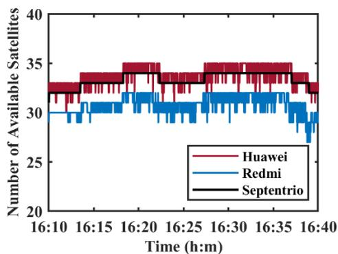
**Figure 7.** The time series of the number of available satellites in quad-constellation.
