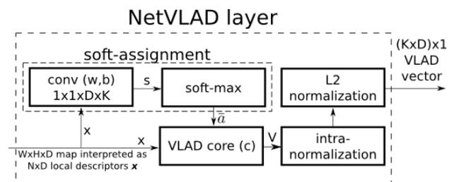
Figure 4. Architecture of NetVLAD Network
