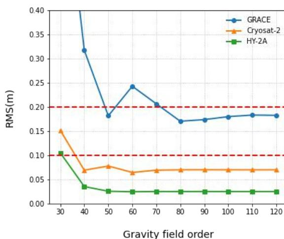
**Figure 5.** RMS(m) in radial direction for different orders in 30 minutes prediction.
