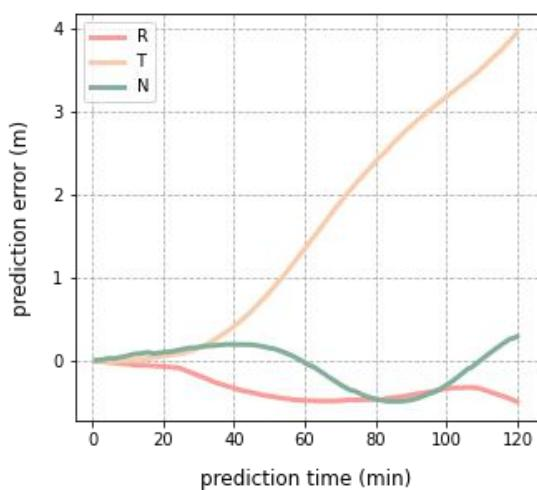
**Figure 2.** Prediction error in 3 directions of GRACE in 120 minutes prediction.
