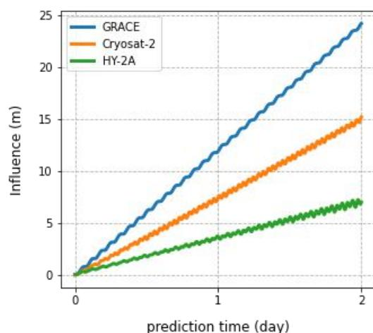
**Figure 7.** The influence of permanent tide on 3D prediction error of different satellites.
