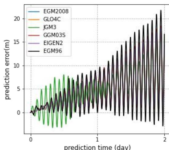
**Figure 4.** The GRACE satellite orbit prediction error (radial direction) in 1st Jan 2012.
