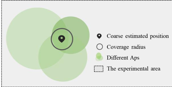
**Figure 5.** Coarse localization: the light grey rectangle represents the entire testing area, the different colored circles represent different APs, the black position is the coarse estimated position, and the black circle indicates the fingerprint matching area.
