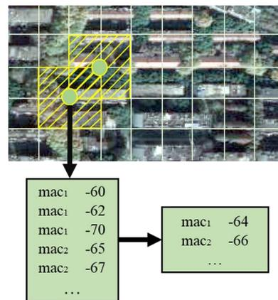
Figure 4. The method of building grid fingerprint database
