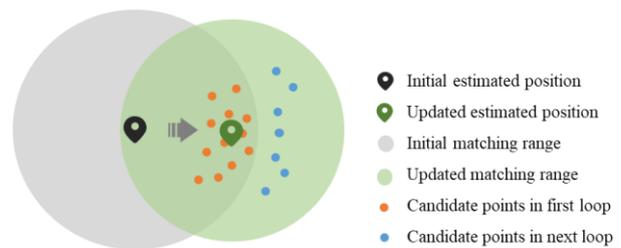
**Figure 7.** The process of iteratively updating the matching area
