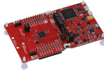
**Figure 2.** SimpleLink™ multi-standard CC26x2R wireless MCU LaunchPad™.
