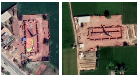
Figure 3: (a) Target map of brick kilns, HR image of the (b) Red and (c) Yellow marked locations respectively showing true positive detections.
