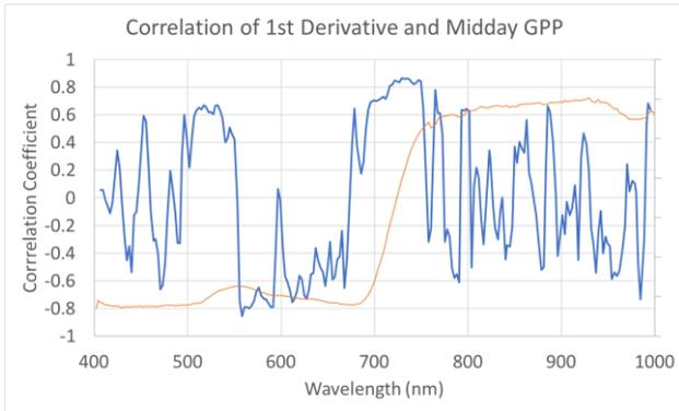
**Figure 7.** Correlations of the first derivative of the DESIS reflectance spectra compared with midday GPP from flux towers. Blue line shows the correlation values, orange line is a representative reflectance spectra (not scaled to y-axis) for orientation.
