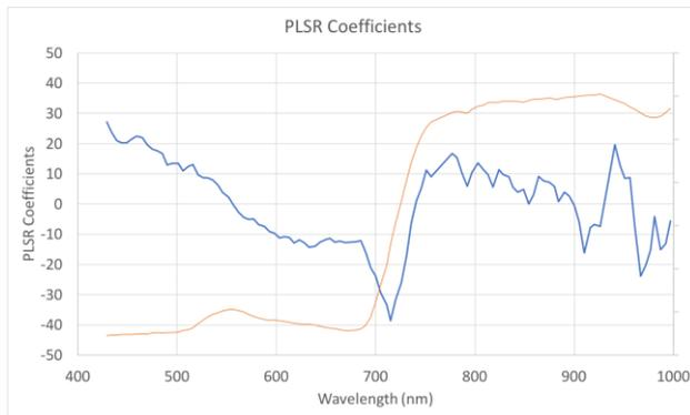
**Figure 11.** PLSR coefficients using DESIS reflectances applied to midday GPP from flux towers. Blue line shows the coefficient values, orange line is a representative reflectance spectra (not scaled to y-axis) for orientation.
