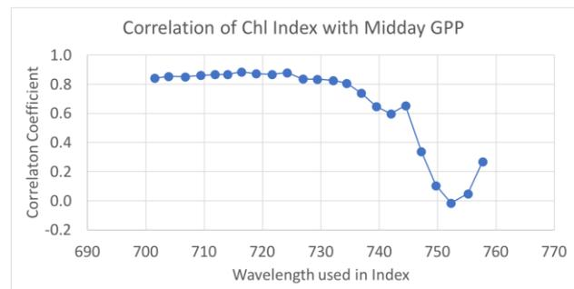
**Figure 5.** Correlation coefficients between midday GPP and the chlorophyll index ( $C_i$ ) using different wavelength bands for the red edge wavelength in Eq. 4.
