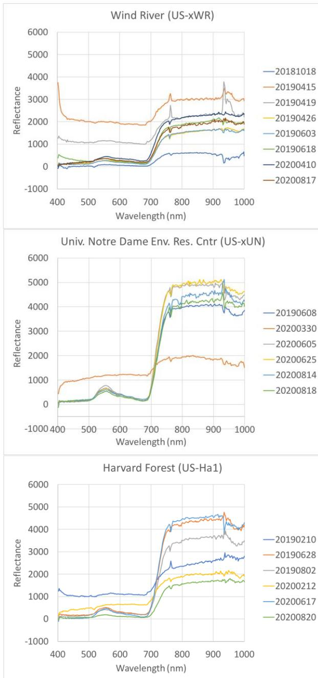
**Figure 2.** Average DESIS surface reflectance spectra for areas around flux towers. The y-axis units are reflectance \* 10<sup>4</sup>. Observation dates are given in the legends in the format YYYYMMDD. Upper plot shows data for Wind River Experimental Forest (US-xWR), the middle plot has data for University of Notre Dame Environmental Research Center (US-xUN), and the bottom plot shows data for Harvard Forest (US-Ha1).
