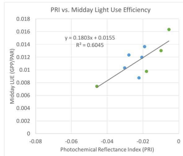
**Figure 4.** PRI from DESIS compared with midday photosynthetic light use efficiency (GPP/incident PAR) from flux towers for summertime deciduous site observations. Blue points are for US-xUN, and green points are for US-Ha1 observations.
