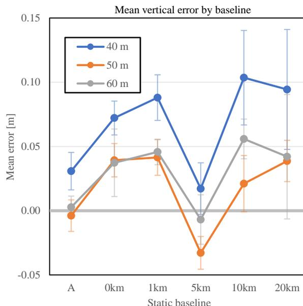
Figure 5. Mean vertical error by baseline. The error bars indicate standard deviation.
