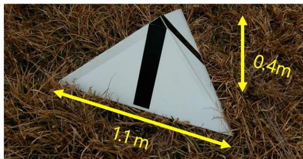
Figure 2. The geometric targets with approximate dimensions when deployed (figure courtesy Wilkinson et al., 2019).
