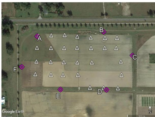
Figure 1. Overview of study site. Control points A-F (magenta) labelled, and target locations shown as white triangles. The area in the southeast corner was avoided so as not to disturb another experiment in progress. (Base imagery courtesy Google Earth)
