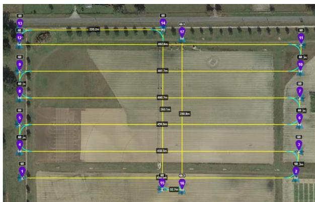
Figure 3. Overview of the 60 m AGL flight plan.
