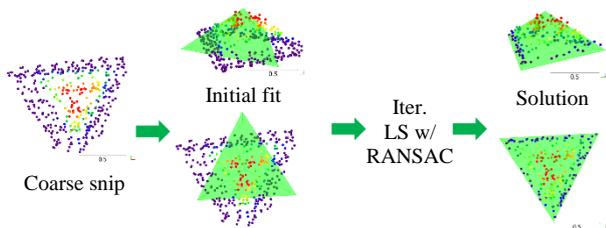
Figure 4. Overview of the pyramid template fitting algorithm.
