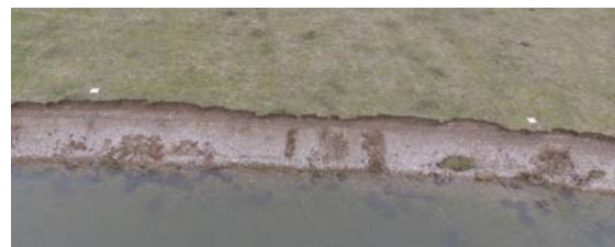
Figure 3: Bank morphology and coded targets as GCPs
