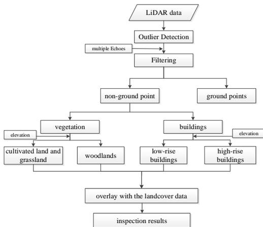
**Figure 1.** The flowchart of the quality inspection of land cover with LiDAR
