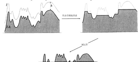
Figure 3. Figure of data filtering based on morphological reconstruction (Cited from literature Lantuejoul C,1984)
