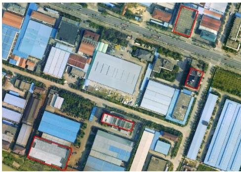
(c) Figure of the buildings that was misclassified to low-rise buildings checked by the Lidar points
