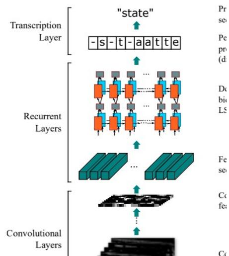
Figure 5. The network architecture of convolutional recurrent neural network for recognizing scene text. The architecture consists of three parts: 1) convolutional layers, which extract a feature sequence from the input image; 2) recurrent layers, which predict a label distribution for each frame; 3) transcription layer, which translates the per-frame predictions into the final label sequence (Shi et al., 2016).
