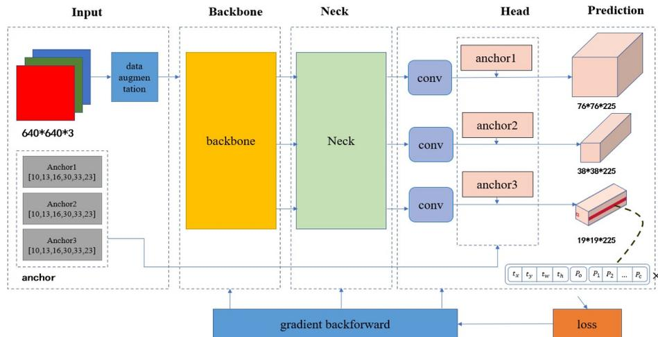
Figure 4. The network structure of the YOLO algorithm.
