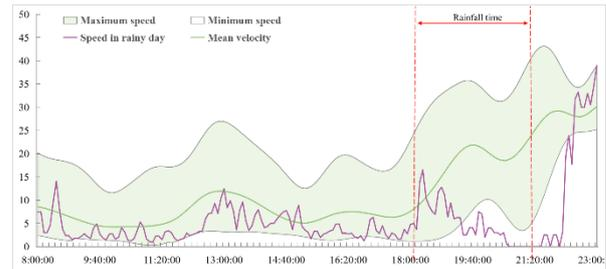
Figure 3. Comparison of road speed (From 8 a.m. to 11 p.m.)
