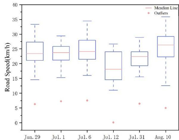
Figure 4. Box plot test of the Zhongyang road speed in rainfall events
