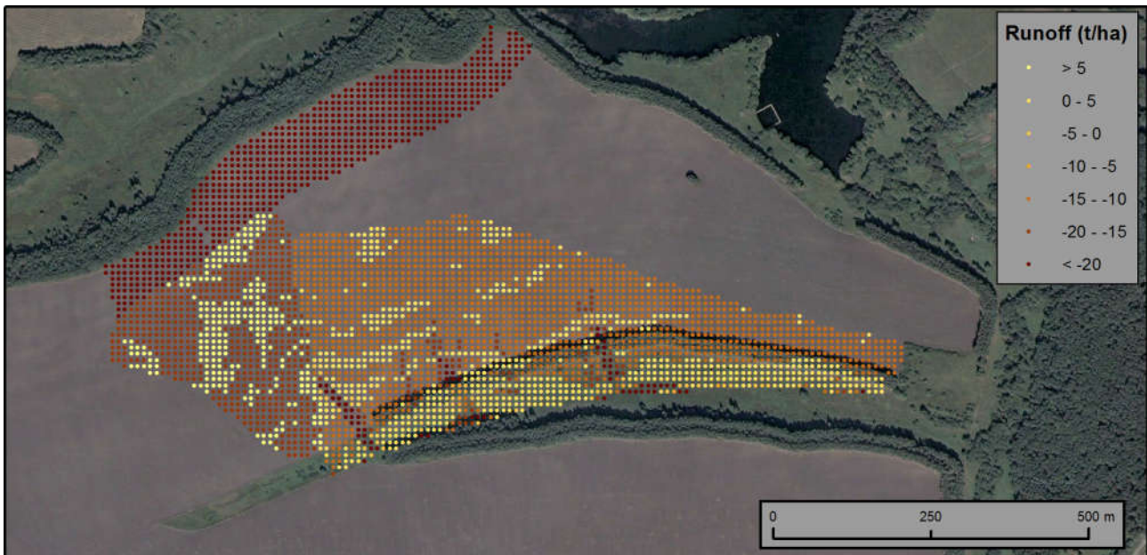
Figure 9. A map of the runoff/accumulation intensity, estimations based upon the dependences of the caesium-137 activity on the catchment area and the sign of the profile curvature. Satellite image courtesy of DigitalGlobe Foundation.
