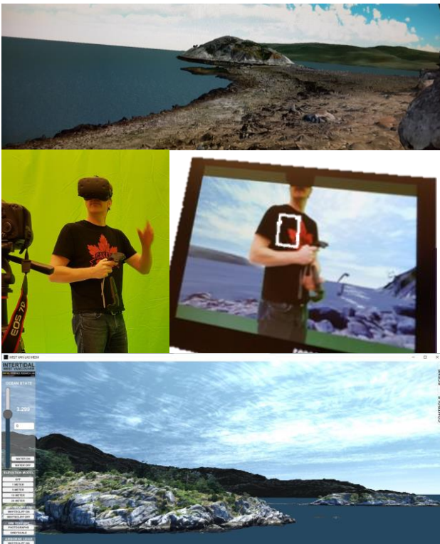
Figure 4. Views from inside and outside of Intertidal VR – and immersive virtual reality system allowing municipal planners and citizens to walk around a 1cm-resolution virtual intertidal space, and interactive control total sea-level (with segmented mean sea-level, storm state), and not just observe, but experience its potential impact on a familiar community coastal space.
