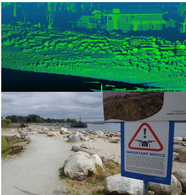
Figure 1. Images from our data survey campaign. Top: view of raw point cloud captured during terrestrial laser scanning of intertidal beach environment. Bottom: in partnership with local municipality and with authorization from federal aviation authorities, we conducted airborne imaging, which we processed using Structure-from-Motion methods.
