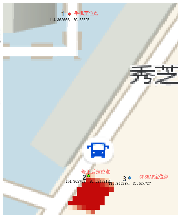
Figure 5. The distribution of the positions located by different methods. The point 1 is the position located by mobile phone, the point 2 is the paper-revised location, and the point 3 is the position located by GPSMAP.
