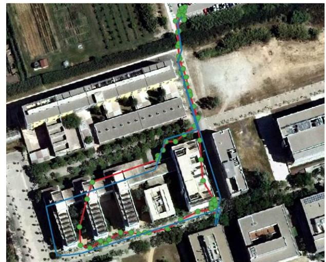
Figure 5. The actual path is shown in blue while the path connecting GNSS locations (green points) is depicted in red.
