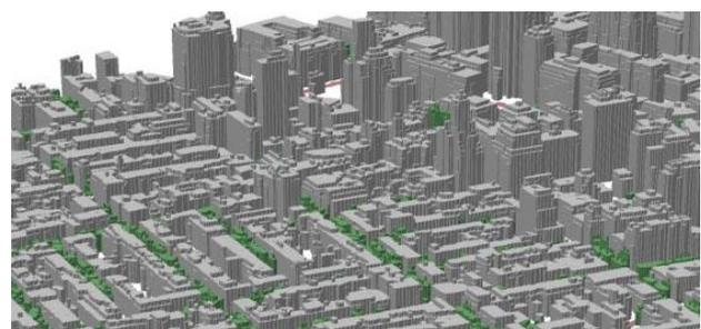
**Figure 3.** Automatically reconstructed building models of Manhattan area using CNN (Agoub et al., 2019)
