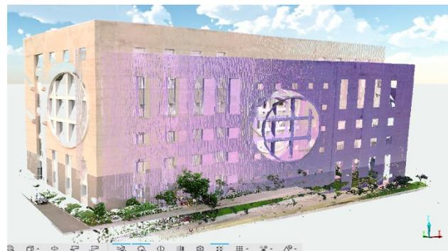
Figure 11. 3D point cloud RGIPT Academic building 2 process data by SCENE software
