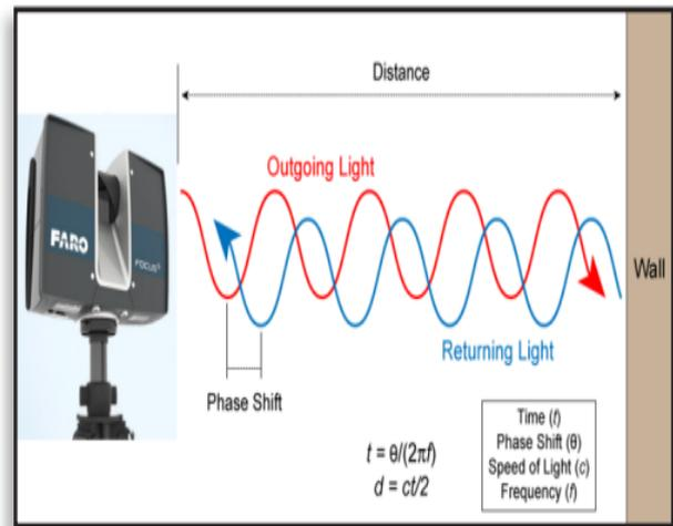
Figure 5(a). The working principle of Phase-based measurement.
