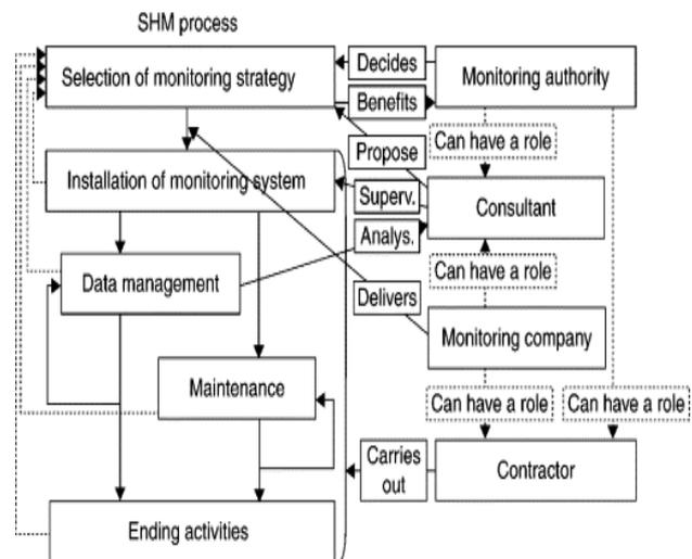
Figure 1. Flow chart for structural health monitoring
