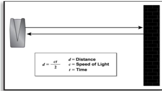
Figure 4. The working principle of time-of-flight measurements
