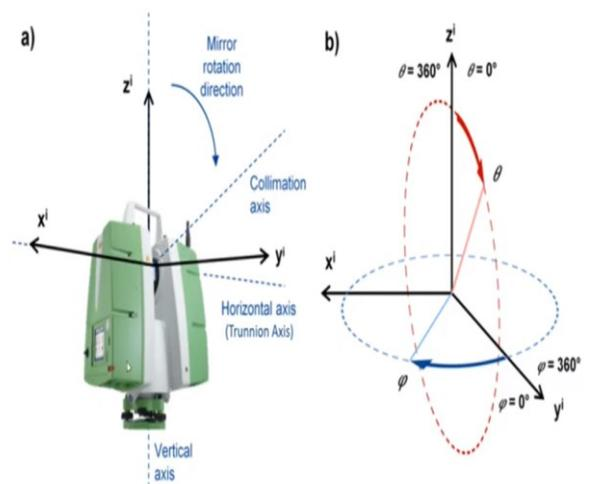
Figure 6. Terrestrial Laser Scanning Axes with their respective angles.
