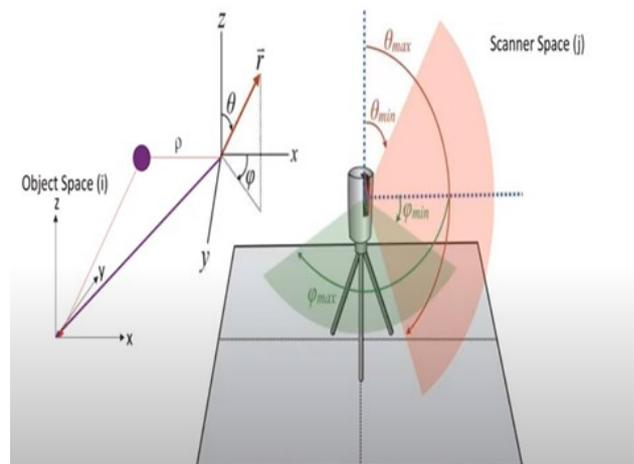
Figure 5(b). The working principle of Phase-based measurement.
