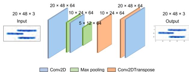
**Figure 4.** Architecture of the autoencoder. The output shape of each layer is also presented.
