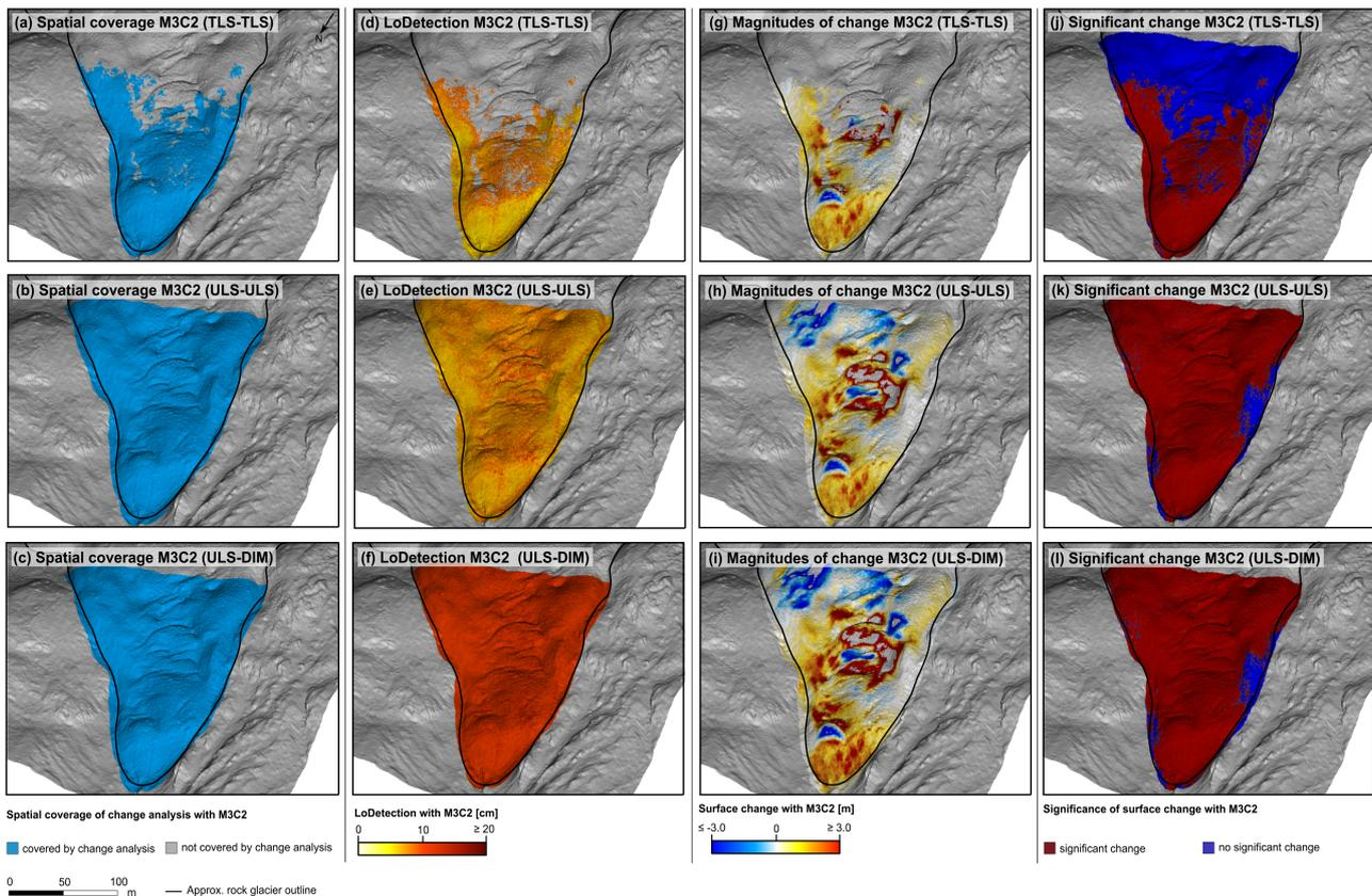
Figure 2. Results of M3C2-based change analysis using point clouds derived from terrestrial laser scanning (TLS), UAV-borne laser scanning (ULS), and UAV-borne photogrammetry using dense image matching (DIM) as input. Spatial coverage (a) - (c), LoDetection (d) - (f), magnitudes of surface change (g) - (i), and significance of surface change (j) - (l) are shown on top of a hillshade derived from airborne laser scanning data.
