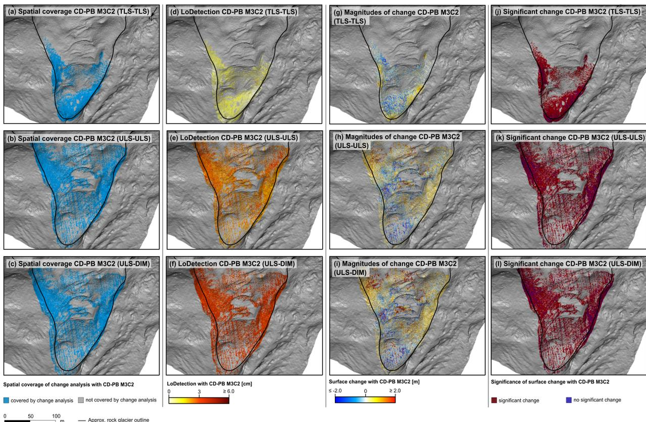
Figure 3. Results of CD-PB M3C2-based change analysis using point clouds derived from terrestrial laser scanning (TLS), UAV-borne laser scanning (ULS), and UAV-borne photogrammetry using dense image matching (DIM) as input. Spatial coverage (a) - (c), LoDetection (d) - (f), magnitudes of surface change (g) - (i), and significance of surface change (j) - (l) are shown on top of a hillshade derived from airborne laser scanning data.
