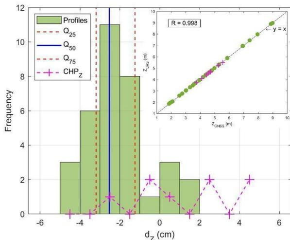
**Figure 3.** Differences in elevation between points measured in the GNSS survey and the elevation obtained UAS DSM.  $Q_{25}$ ,  $Q_{50}$  and  $Q_{75}$  are the quartiles of deviations in profiles points. The plus-dash line illustrates the histogram of  $CHP_z$ . In the top right is represented the linear regression of the vertical position. Circles correspond to P and plus sign correspond to  $CHP_z$ .
