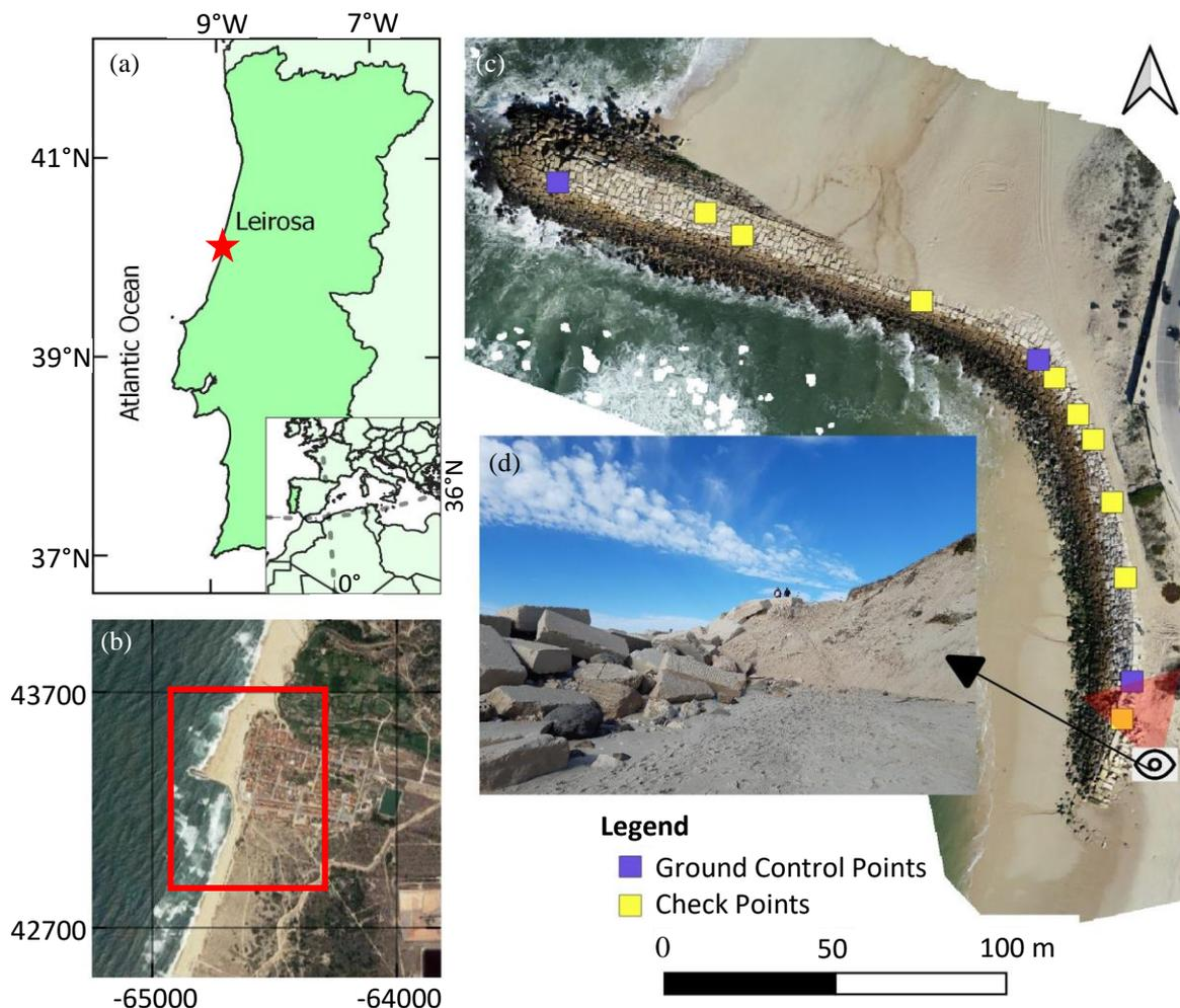
**Figure 1.** Study area illustration. (a and b) Location of Leirosa Beach in the Portuguese coast (red star in (a) and red rectangle in (b)). (c) Orthophoto generated by drone survey of Leirosa groin. The colored squares represent the control points used in the photogrammetric process. (d) Photo of the south groin head showing several blocks displacements.
