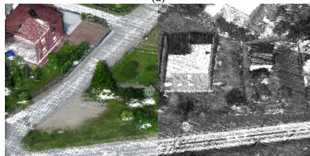
Figure 4. Part of UAS LiDAR point cloud collected in 2018 (a), and in 2019 (b). Left – colored by RGB data. Right – shown in greyscale intensities.
