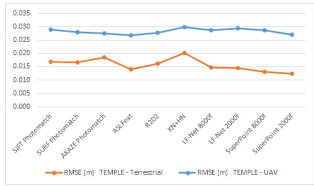
**Figure 6:** RMSE [m] for the *Neptune Temple* datasets. In both cases (terrestrial and UAV), the RMSE variation is very limited, the different methods behave in a similar way, especially in the UAV dataset where the sensor-object distance is very high.
