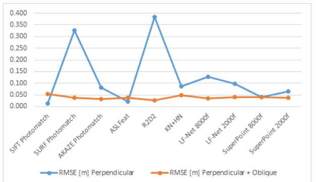
**Figure 8:** RMSE [m] for the *Paestum Wall*. SURF and R2D2 produced a pronounced curvature/deformation - not visible from the MRE analysis – in case of only perpendicular images. The use of oblique images reveals a minimal RMSE differences between the various methods.
