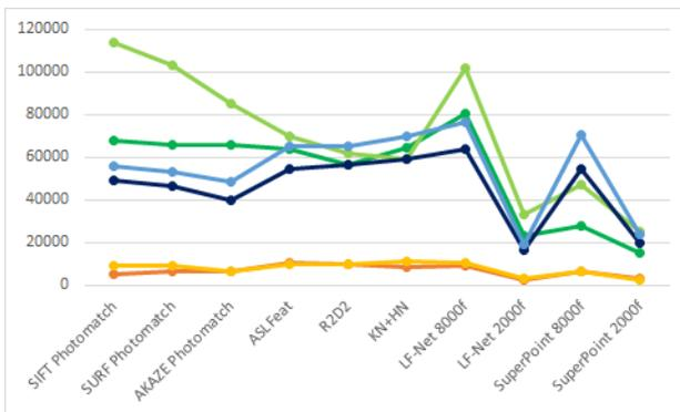
**Figure 5:** Computed 3D points (sparse cloud) within the bundle adjustment. In *Paestum Wall Perpendicular + Oblique*, ASLFeat, R2D2 and Key.Net+HardNet methods, having a higher MTL, create significantly fewer 3D points.
