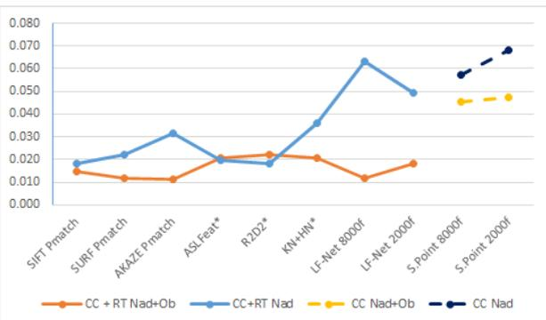
**Figure 7:** RMSE [m] for the *Ventimiglia Theatre* dataset, with only nadir images (*Nad*) and with the inclusion of oblique images (*Nad+Ob*). The SuperPoint tests are performed with only cross-check (CC) instead of cross-check + ratio test (CC+RT).
