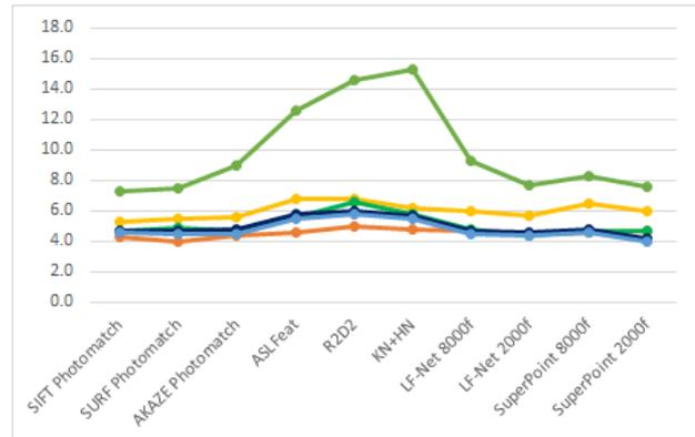
**Figure 4:** Average MTL for extracted tie points. ASLFeat, R2D2 and Key.Net+HardNet always show a higher MTL value with respect to the other learning-based methods.
