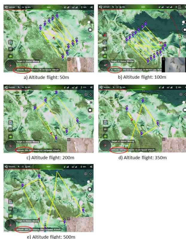
Figure A1: The five missions' plans at different altitudes
