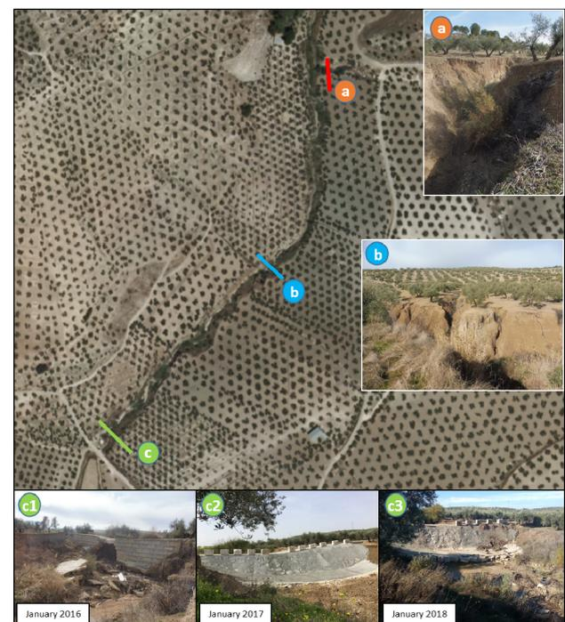
Figure 2. Photographs of different sectors of the gully area. (a): V-shape of a section at a tributary gully. (b): soil slab fall at the steep sidewalls. (c): Damages affecting a rural path due to upstream erosion from 2016 to present.
