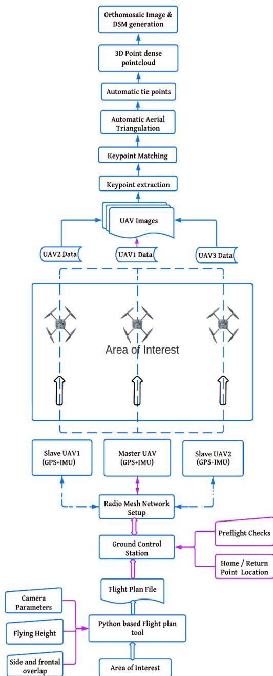
Figure 8. Complete methodology for UAV swarm system for aerial mapping.
