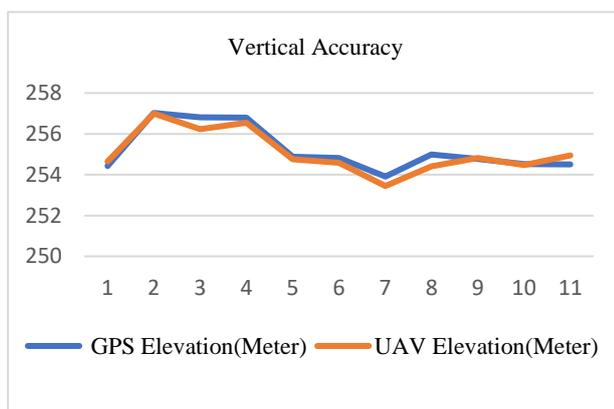
**Figure 11. Comparison between GCPs and derived corresponding elevation values**
