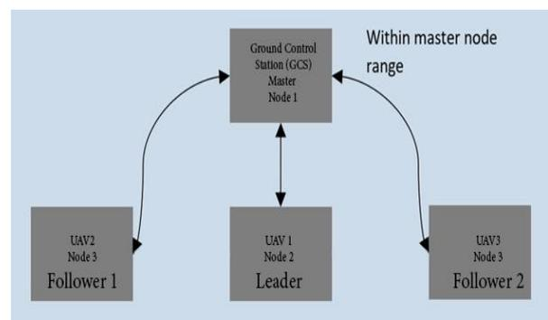
**Figure 4. Multipoint mesh network using RFD900x modules.**
