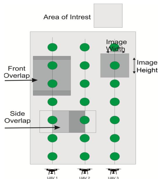
**Figure 7. Flight parameters for UAV swarm flight.**
