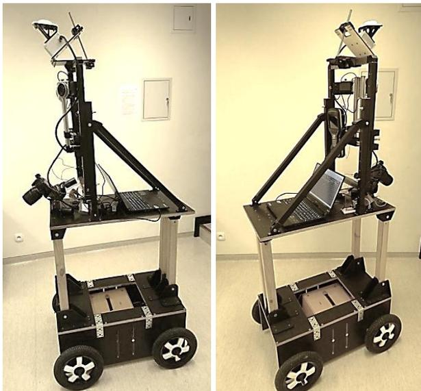
Figure 1. The prototype of the platform with integrated sensors
