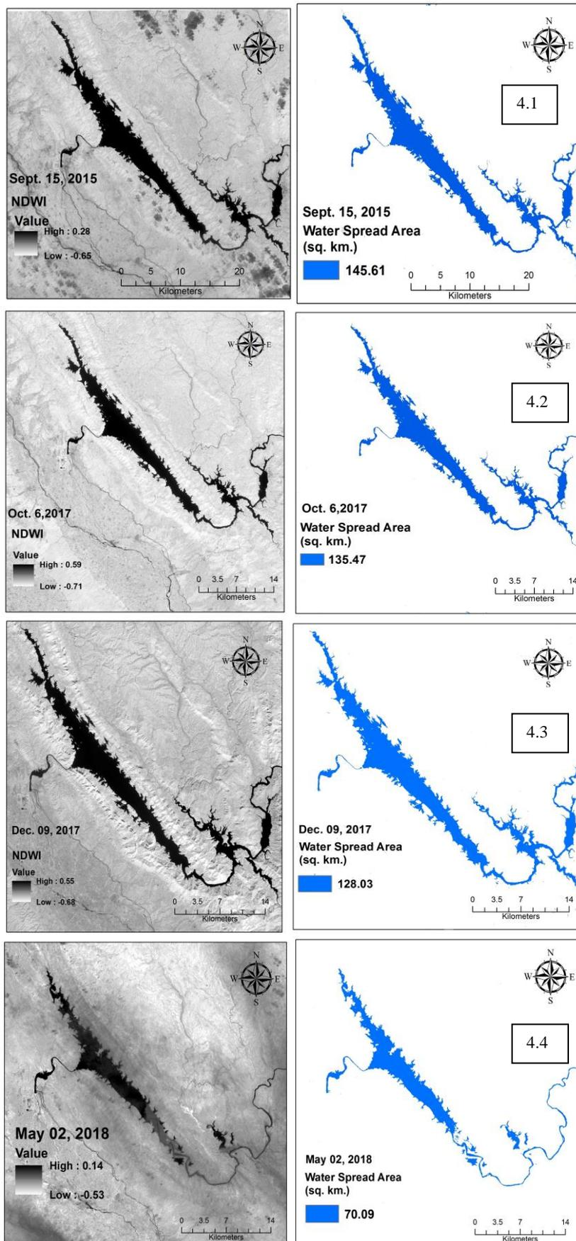
Fig. 4.1 to 4.4 NDWI map of different dates obtained from Google Earth Engine and corresponding masked water pixel.
