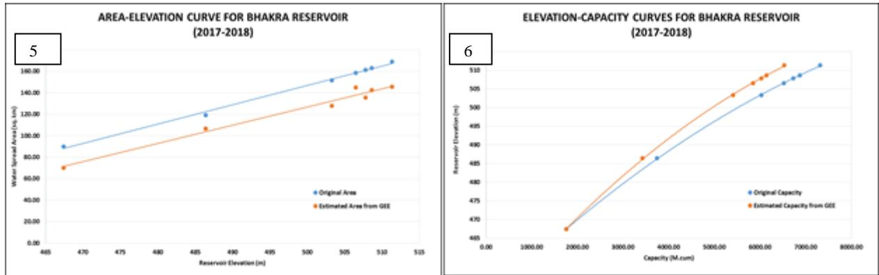
Fig. 5 Elevation-Area curves for Gobind Sagar Reservoir, India (2017-2018)
