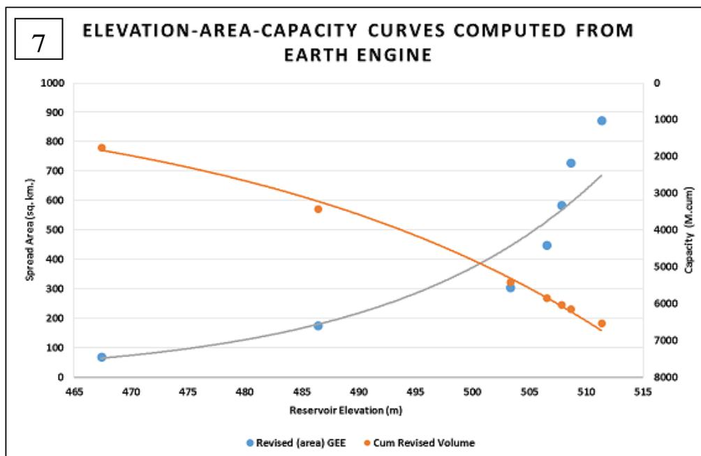
Fig 7 Elevation-Area-Capacity curves for Gobind Sagar Reservoir, India (2017-2018)
