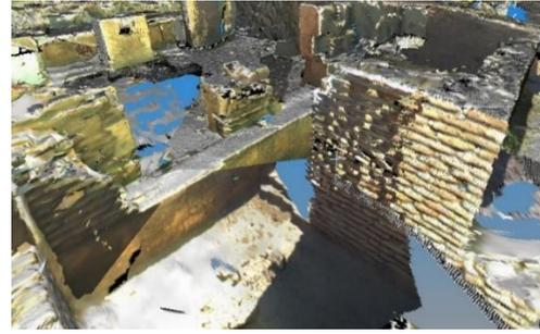
Figure 5. Point cloud after meshing
