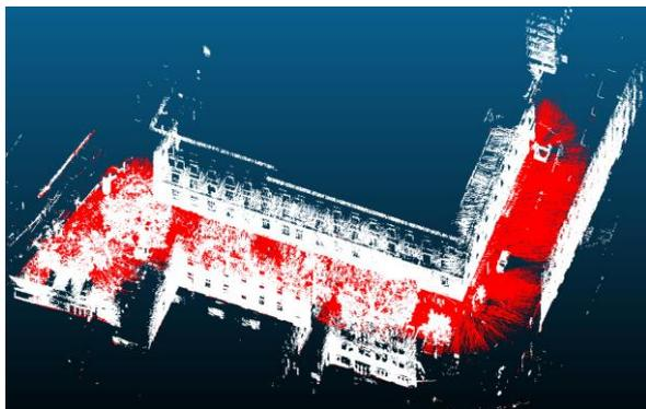
Figure 4. ground and non-ground points which are separated in white and red colors respectively
