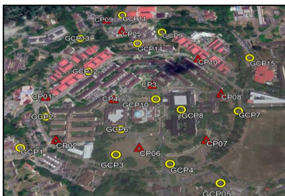
Figure 2: Location of GCPs (yellow circle) and CPs (red triangle) in the study area.
